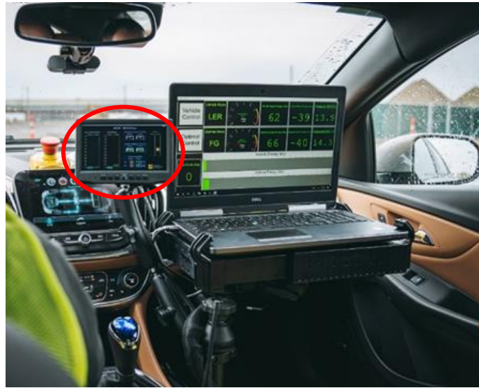
Figure 3.1 HMI display (circled) positioned in the front passenger seat of the vehicle.
